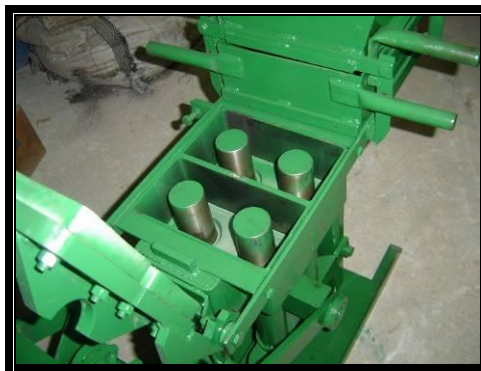
MOULE STABI-12 Installé
